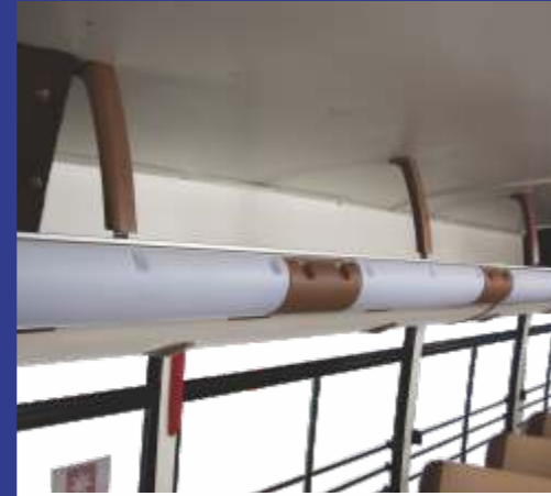
Modular hatrack with integrated AC duct
