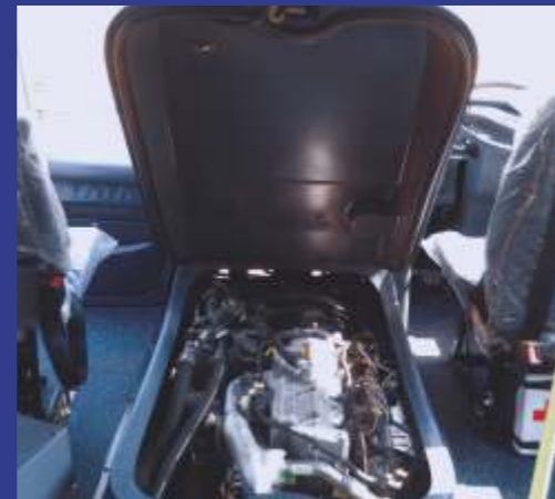
Special heat and noise insulation in the engine hood
